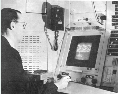
Ivan Sutherland, SketchPad, 1963, MIT CRT, light-pen, direct-manipulation 2D graphics
